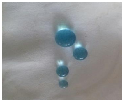
Figure 4. Water droplets on super hydrophobic titania hybrid coated a) fabric b) paper.
